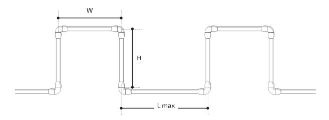
Long straight pipes will expand or contract due to temperature variations. To compensate for this effect, expansion loops are required. The number of expansion loops depends on the total length of the straight line and the maximum temperature variation. An expansion loop is a U-shaped construction that compensates the variation in length.
