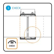
Note: When replacing the old D100 fitting with the new D100 fitting, only a new marking is needed, no cutting of pipes.
